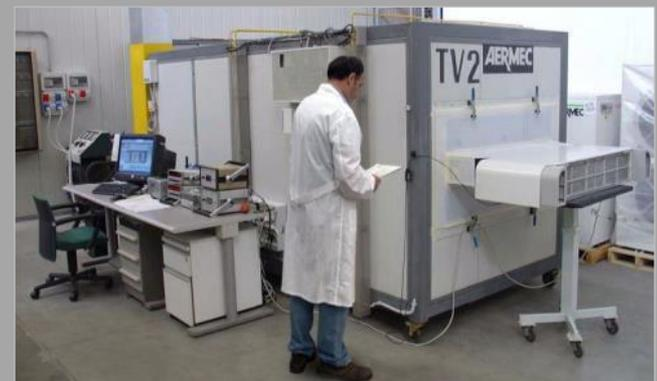
fan coil performance test simulator
